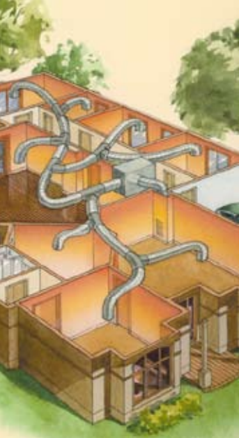
SIMPLE, BUT CLEVER: A mechanical ventilation system can make a huge difference to the temperature of your house, while (right) a heat exchanger
