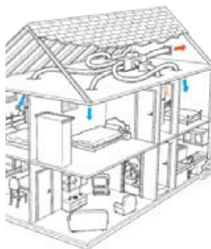
LOFTY AIR CON: Utilising the attic
